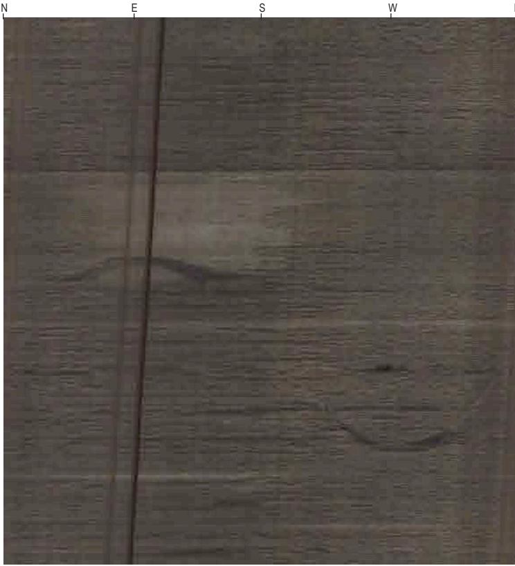
Horizontal Fracture Lower Huron Shale
